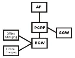
Fig: Interactions of PGW with PCRF, and Charging.
