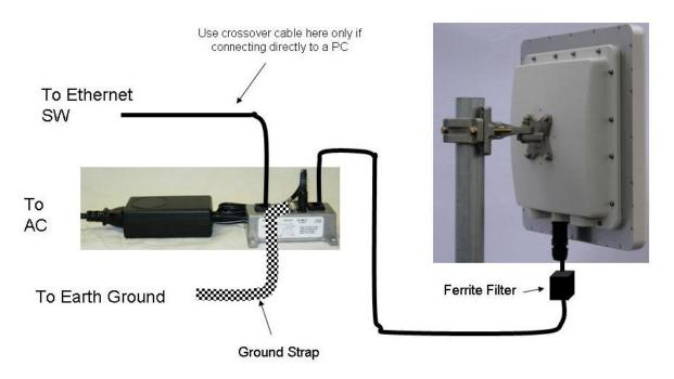
Figure 1 Connection Diagram
